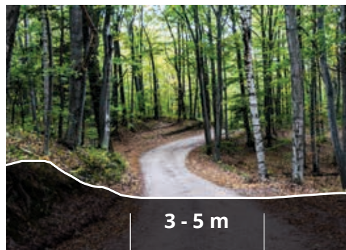
Multi Use Trail, Typical Crushed stone granular surface
