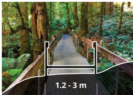
Raised Boardwalk, Guided Wire Mesh/Wood Surface
