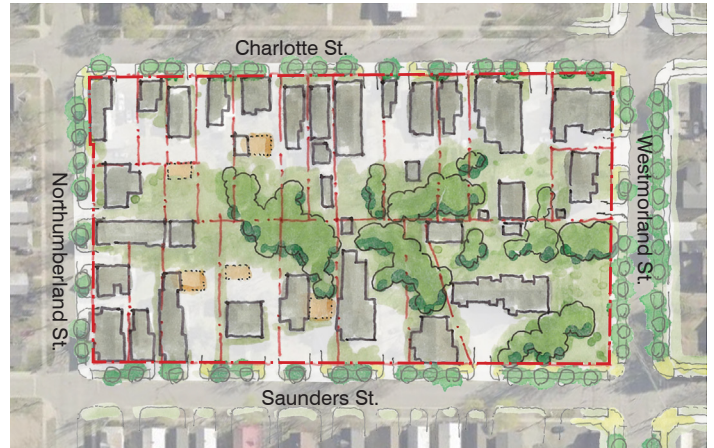
Demonstration illustrating secondary dwelling units located to preserve the permeable "Sponge Area" at the rear of lots
