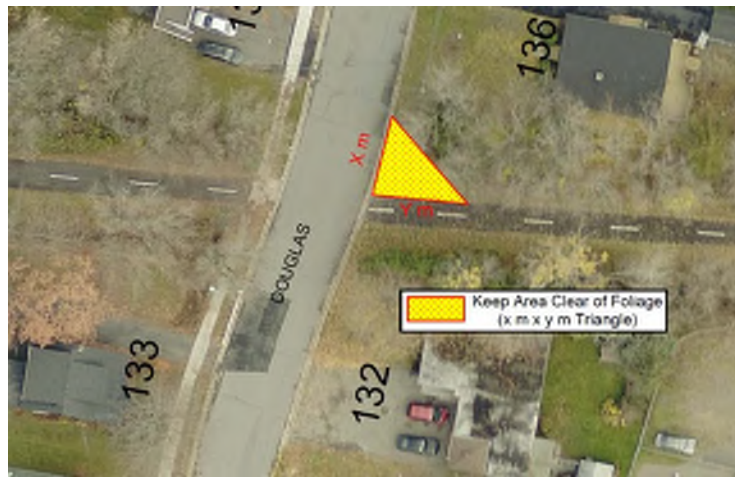
Figure 12: Sight Triangle Example
