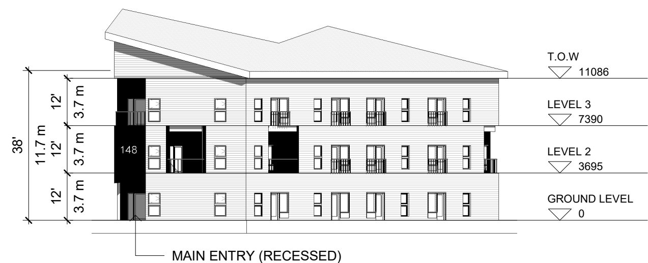
ENTRY ELEVATION (CLARK ST.) 1 : 300
